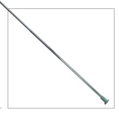
ALUMINIUM TUBE BD 1000-1900 MM Adjustable aluminium tube, with bolt on top (Ø 10 mm) to take T-piece, mounted with tube holder in white, silver-grey or black. Suitable only for BD bases Ø 255 mm and Ø 345 mm. Inner tube Ø: 16 mm, outer tube Ø: 20 mm.
